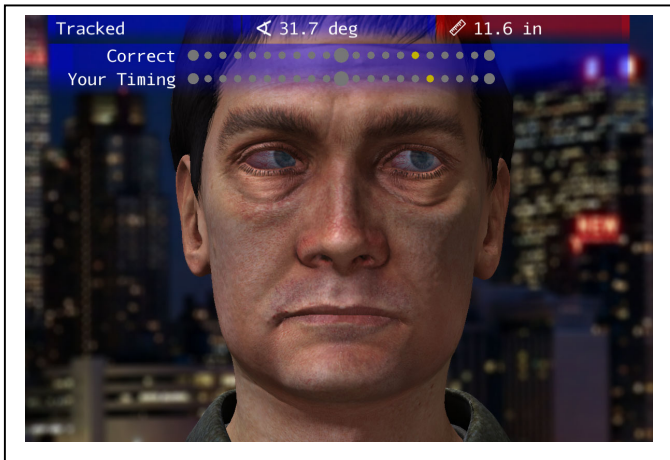
Fig. 5. The motion stats display the angle and distance of the user's finger relative to Brian. The visual metronome enables trainees to see live feedback about the speed and timing of their finger/stylus movement.
